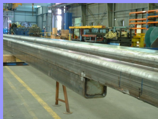
Side Sills being Rollformed & Assembled manding build schedule.
