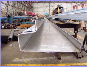
Cant Rails being Rollformed & Packed for Despatch
