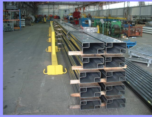
Cant Rails being Rollformed & Packed for Despatch
