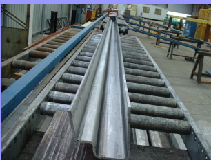
Side Sills being Rollformed & Assembled manding build schedule.
